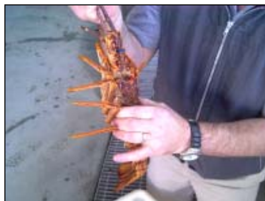
Figure 3. Processor testing for shell hardness by squeezing along the lateral suture which runs down the side of the carapace. This region of the carapace was targeted in durometer trials (locations 4 and 5).
