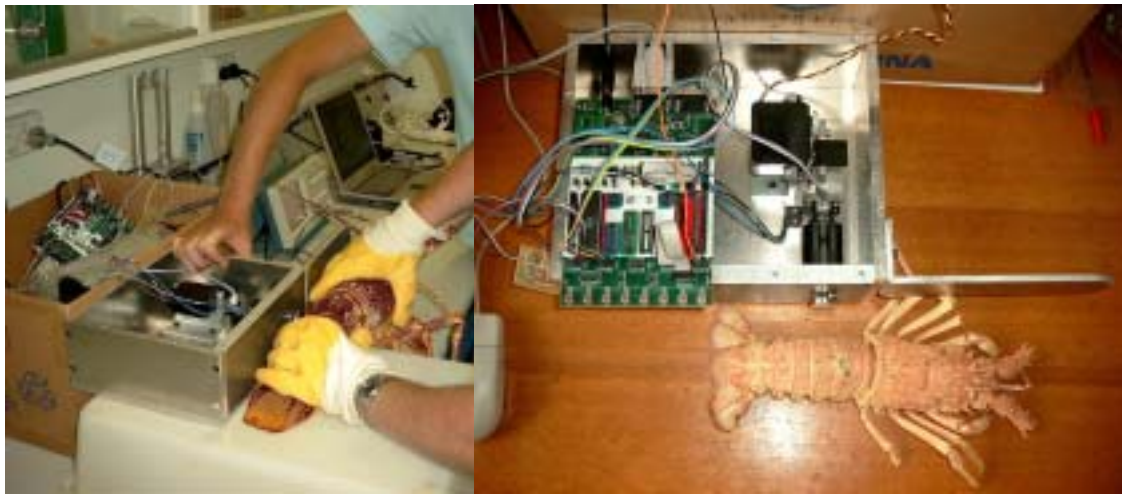
Figure 23. Prototype gauge to measure lobster shell hardness in development. A piston moves out until it touches the surface of the lobster and then moves a further 5 mm. The force that is required to produce this flex in the tail is measured – softer lobsters require less force. Readings are stored in memory for research applications. For industry application, LEDs are illuminated with illumination of all LEDs indicating the lobster is fully hardened.
