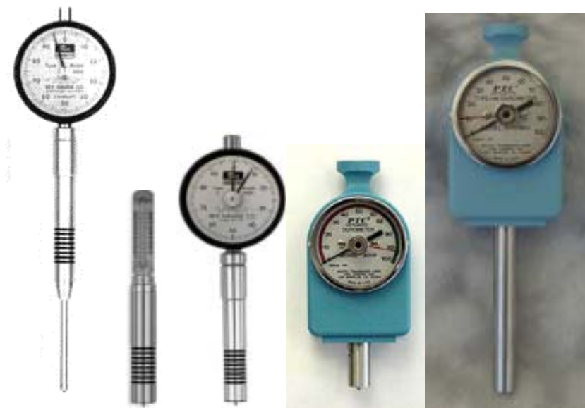
Figure 1. Durometer models. Key differences between models are the size of the foot (4.8 mm or 11 mm) and the display system (either vernier or dial). Durometers come in different grades, depending on the hardness of the material to be measured; most crustacean applications are with A or C grade durometers. The two gauges tested in this project are at left, the Rex 1700™ (narrow foot) and Rex 1500™ (broad foot).
