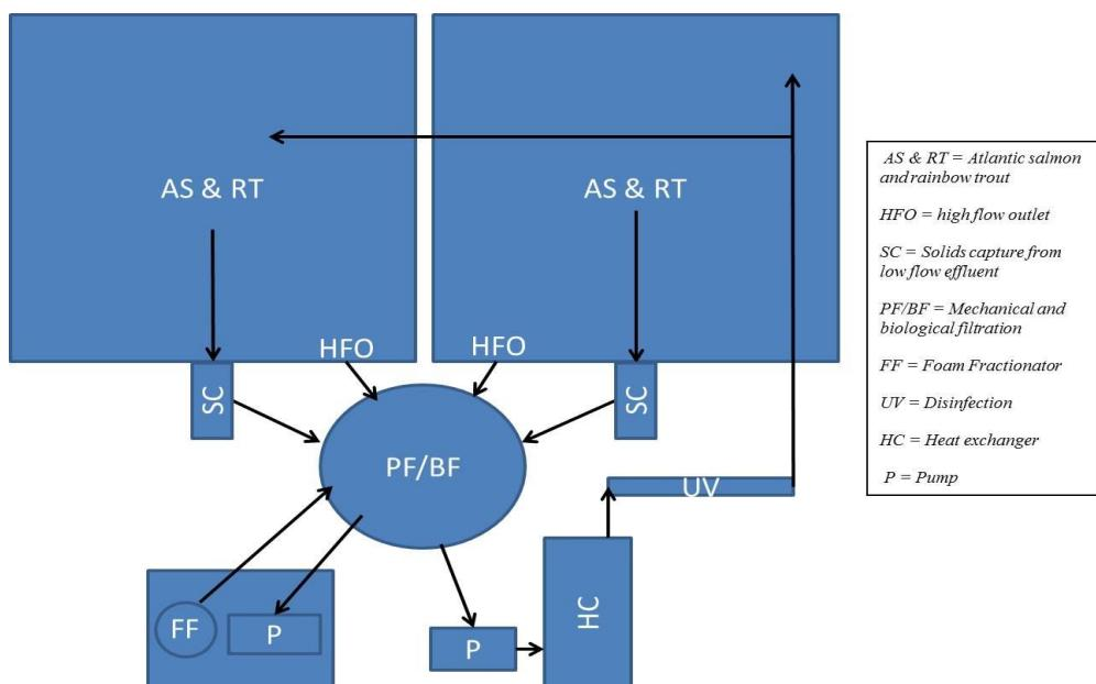
Figure 5. Modified recirculating system configuration used for housing mullet and Atlantic salmon during Experiment 6.
