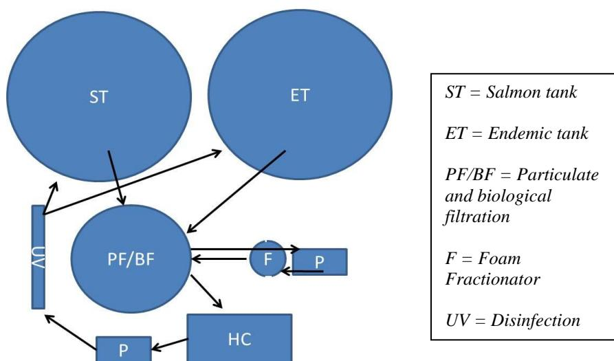
Figure 2. Recirculating system configuration for experiments 1 – 4.
