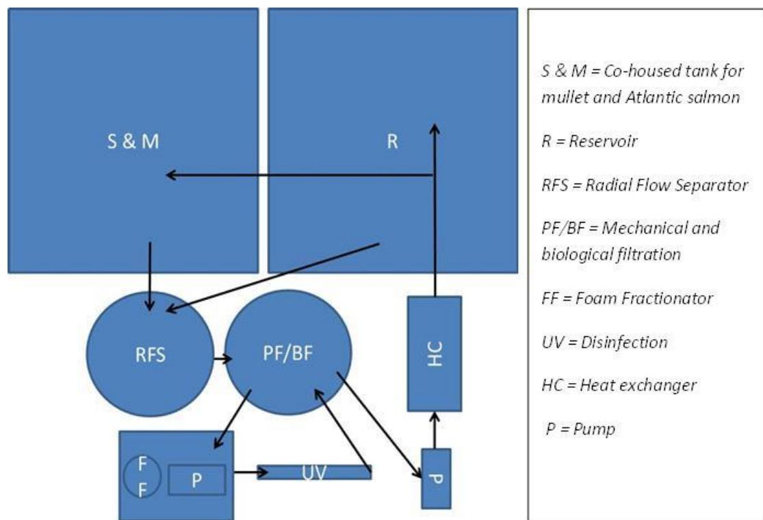
Figure 4. Recirculating system configuration used for housing fish during Experiment 5.
