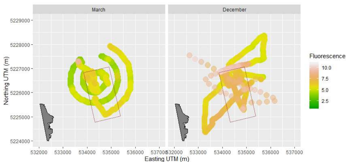
Figure 3-14: Heat maps produced from continuous sampling of surface water column for fluorescence ( \text{mg}/\text{m}^3 ) collected by the DUDES sampling system in both March and December 2021.
