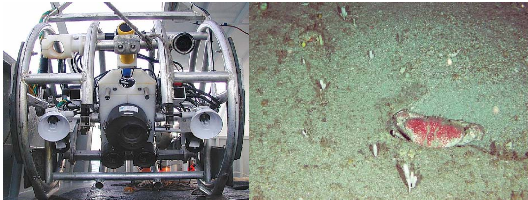
Figure 22. Deep water video system used for collecting images of giant crab habitat and a male giant crab encountered on the first survey at around 300 m.
