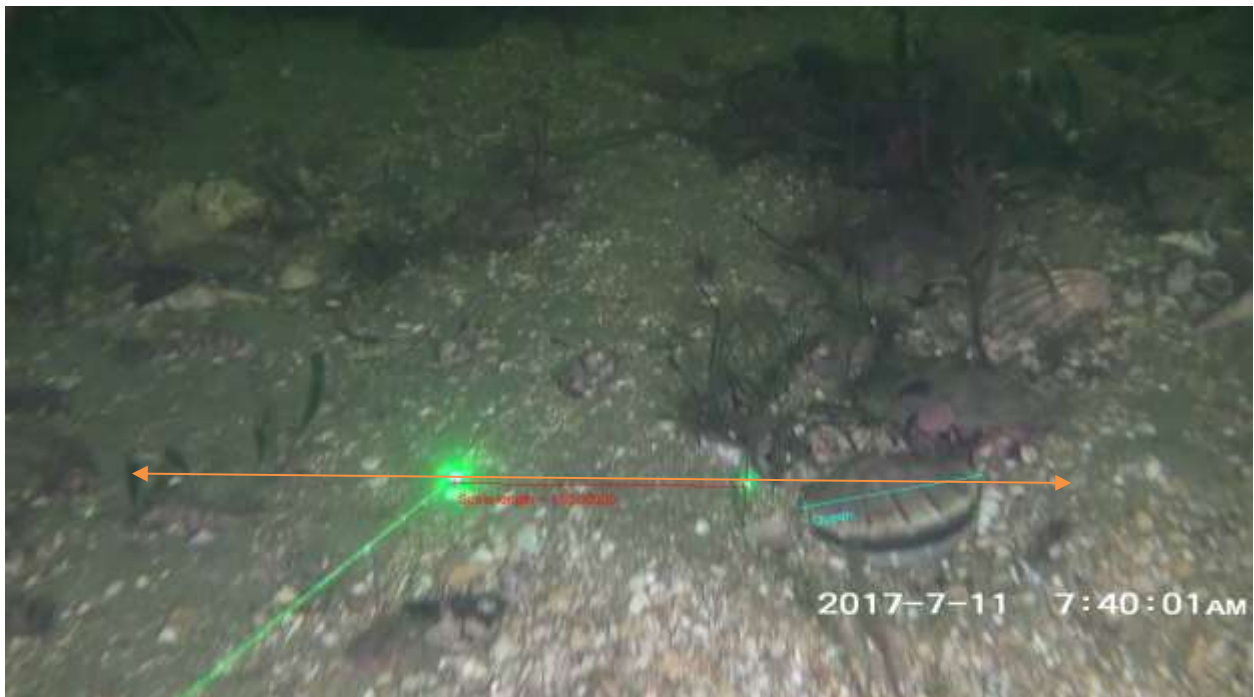
Fig. 3: Frame from video footage showing scaling lasers (green dots), pixel to millimetre calibration (red line), video centre line (orange line), transect width (orange line is 500mm long and centred at the centroid of the scaling lasers), and a scallop width measurement (blue line) orientated at 10° to the centre line.
